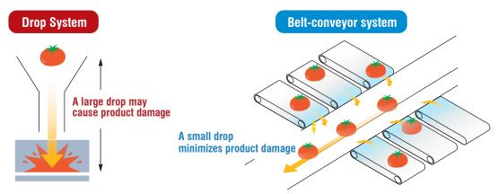
Belt-conveyor system with reduced drop height allows transfer of fragile or sticky products.
